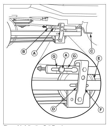
Figure 24. Adjusting Belt Tension
